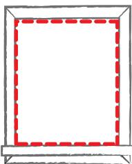
**Inside mount** window treatments are installed inside the window casing.
