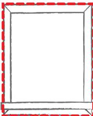
**Outside mount** window treatments are mounted outside the window casing and provide better privacy and light control. They're mounted directly on the wall or the window molding.
