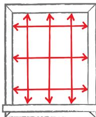
For **inside mounts**, measure the depth of your window frame. Then, measure the inside of the frame in three places for width and height.
