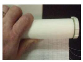
**5.** While keeping the shade completely rolled, reinstall shade starting with control end. Ensure the latch on the non-control end is open, then place into notch, close lever.
