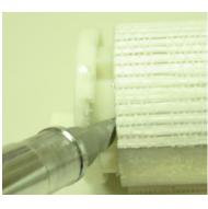
**5.** Insert new clutch and/or idle end into tube by hand or with a mallet until fully seated.
