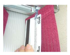
4. Remove the headrail from the mounting brackets by placing the flat head of a screwdriver between the back of the headrail and the release clip on the mounting clip. Pull the handle of the screwdriver toward the front of the rail and tilt rear of the headrail down and toward you. (If you have a curved/bowed headrail, please refer to step #5).
