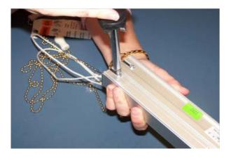
14. If your blind was made after January 2004, follow steps #15 – 18. Lay headrail on a clean flat surface with louver stems pointed away from you. On top of the headrail on the end with control mechanism, locate screws connected to a metal plate.
