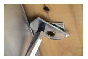
6. If your blind was made prior to January 2004, lay the headrail on a clean flat surface with louver stems pointed toward the ceiling. Inside the headrail next to the control mechanism are screws connected to a metal plate. If your blind was made after January 2004, follow steps #15 - 18.
