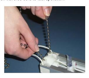
19. Once you have confirmed the headrail is working properly, reinstall the headrail into the mounting clips and reinstall the louvers in the open position as pictured below. All louvers should be facing the same direction.
