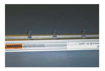
**12.** Turn the headrail over and place the chain over the chain gear making sure the ends of the chain are even.
