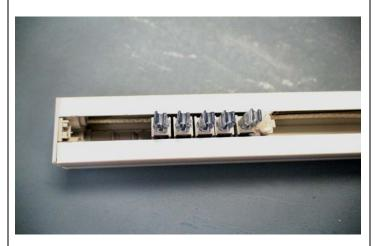
6. To remove the control mechanism end cap, place thumbs on the end of the end cap at chain/cord opening. Push firmly against the end cap edges and push the sides of the end cap away from the headrail. The end cap will slide off once the sides release from the housing.
