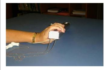
14. To insure that the control end has been installed correctly, rotate the stems open and closed several times by pulling the rotation chain and slide the carriers back and forth several times by pulling the traverse cord.
