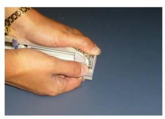
7. If the small gear inside the housing is missing or stripped, replace it with the new gear included with the parts sent to you.
