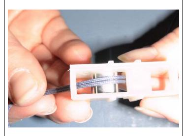
**8**. Turn cord lock upside down. Place the rivet inside the new cord lock. Make sure the cord is between the rivet and smooth roller.
