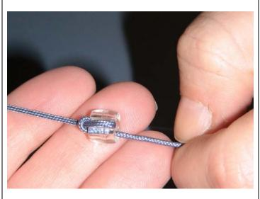
**18.** If the stop beads ARE NOT 2" to 3" below the headrail, loosen (but not untie) the knot surrounding the bead.
