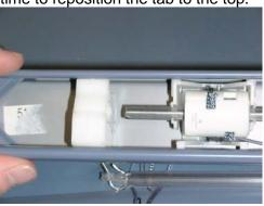
7. Keeping the blind level, reinsert the tilt rod.
