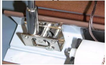
**8.** Thread the cords under the side of the new cord lock, over the smooth roller, and between the smooth and the serrated roller.
