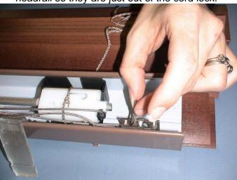
7. Place a flathead screwdriver inside the cord lock and push towards the back of the headrail. The cord lock should disengage.
