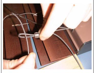
20. Confirm the stop bead is located 1 to 2" below the headrail. Push the cord into the groove on the side of the bead and tighten the knot firmly. Pull the knot inside the stop bead. Repeat for the second bead.
