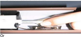
15. Replace the end caps. Use rubber mallet if necessary to ensure a tight fit.
