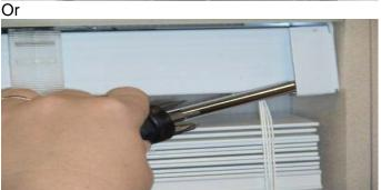
3. Remove the cord tassels, washers, and cord stop beads from the lift cords and set aside. If the blind has more than 2 cords, the stop tassel will need to be removed and the knot untied.
