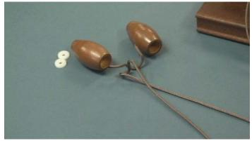
**4.** Remove the end caps by gently tapping with a screwdriver or rubber mallet.
