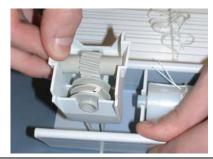
**8.** Slide the tilt rod through the wand tilter. Be sure the tape drums are in the open position before inserting rod.
