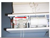
7. Place the new wand tilter into the rail, guiding the stem through the cut out. Push down firmly on the back side until the tilter is in position.
