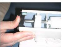
11. Locate the hole at the top of the long groove on the tilter stem and insert the wand connector clip.
