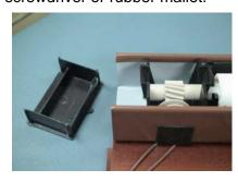
Or remove the blind's end stiffeners with needle-nose pliers.
