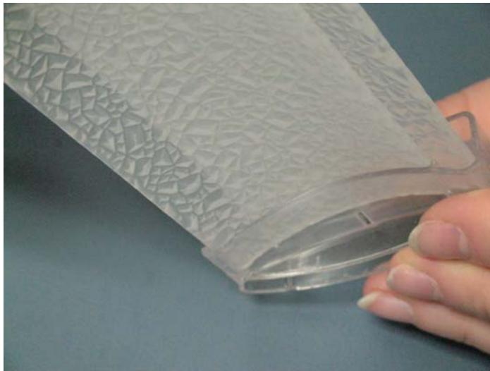
4. Slide the second valance slat into the valance return bracket. The bottom of the slat will be at the bottom of curve.
