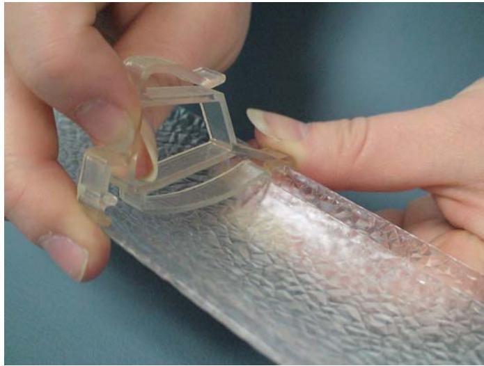
2. Slide the first valance return slat into the valance return bracket. Top of the slat will be at the top of the curve. The return slat will stop at the tab.
