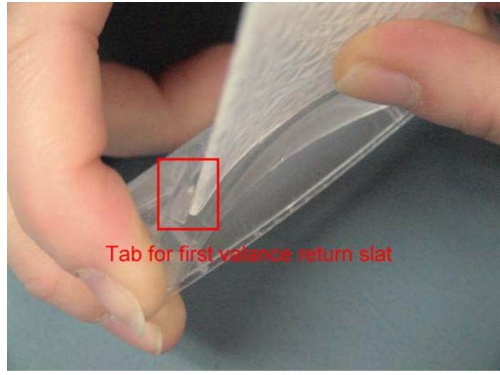
3. Slide the second valance return slat into the valance return bracket. The bottom of the slat will be at the bottom of curve.
