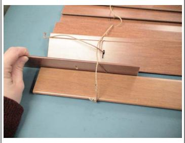
10. After replacing the slat(s), re-thread the lift cords through the rout holes. Make sure to interlace or move the lift cord from the left side of the ladder rung to the right side of the ladder rung every 2 or 3 slats. Continue for all lift cords.
