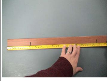
**8.** Continue in the same manner with the remaining rout holes. Record all the remaining measurements. Record the overall width of the slat to the nearest 1/16".
