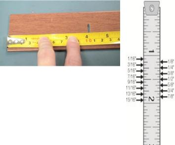
7. With the tape measure still on the left side of the slat, measure the middle of the second rout hole from the left side of the slat. Record this measurement.
