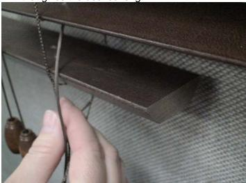
**6.** Thread the lift cord through the hole in the bottomrail.
