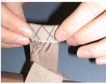
**13.** Insert upholstery tacks into the ends of folds over the retainer button. You may need a small hammer to tap the tacks into the bottomrail.
