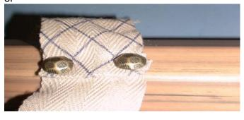
3. Untie or cut lift cords under the retainers. While holding bottomrail, use needle nose pliers to squeeze open the brass crimp (if applicable). Remove brass crimp and retain for later use.
