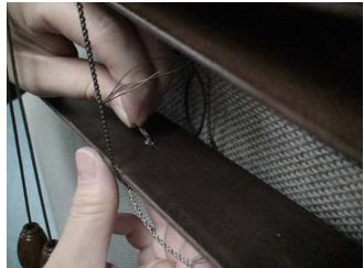
7. Cut off the excess ladder cord. Leave one rung just below bottomrail.
