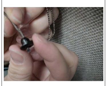
**10.** Cut off excess cord. Tuck brass crimp and ladder cord into the bottomrail hole. Snap retainers into place on the bottomrail.
