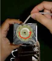
**6.** Reinstall the new continuous cord loop by gently turning and wrapping the loop under the teeth of the clutch.
