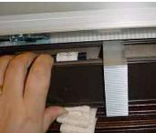
**4.** Set the blind on a flat surface and remove clutch endcap by placing a screwdriver under the lip at the top of the clutch and twist.
