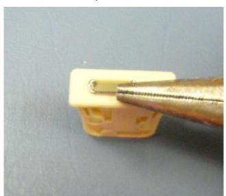
**19.** Feed the cord through the cord lock, making sure the cord is between the silver rivet and the roller in the cord lock.
