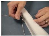
Pleated: Note: For shades with loop tape, be sure the cord is threaded through each loop. Count the number of loops to match the number of pleats.
