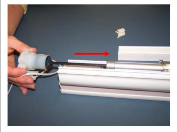
**11.** Reinsert the cord divider into the clutch. Make sure the continuous loop lays in the grooves of the divider. Slide divider up into the clutch.
