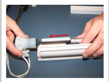
**10.** Reinstall the continuous loop by gently turning and wrapping the loop under the teeth of the clutch.
