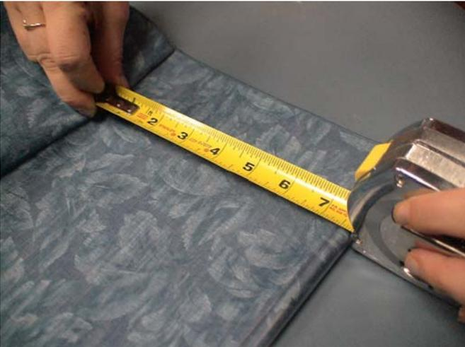
8. Carefully unroll the fabric from the sill rail. Reroll the fabric keeping taut and parallel with the pleat above. Check bottom pleat for evenness by measuring again. Replace sill rail cover.
