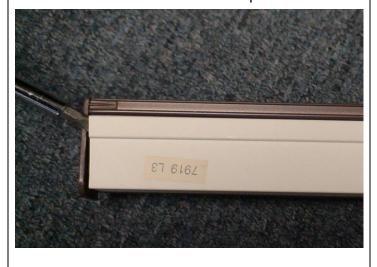
**4.** Manually turn the rod 2 turns toward the back of the shade. Now raise the shade using the handle.
