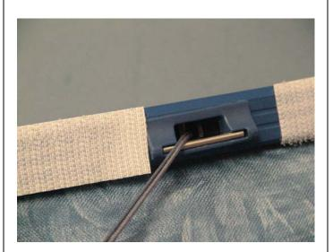
3. Position cord away from cord lock. Insert small screwdriver into black plastic guide. For a left control, slide the black guide to the right. For a right control, slide the black guide to the left. Once done, shade should operate correctly.
