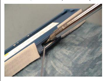
4. If shade still does not operate correctly or remains locked, unscrew bottom joiner ball from top joiner ball with the shade in the raised position. Untie the knot from the cord. Smooth cords between fingers and retie cord into a knot.
