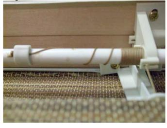
2. Slide cord clips to the left or right along the shaft (while holding the shaft stationary) to correct small discrepancies in cord length.
