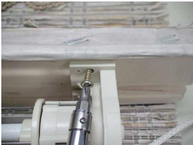
12. Make sure cord clips are evenly spaced from shaft bracket. It is important the lift cord starts on the back line located on the shaft.
