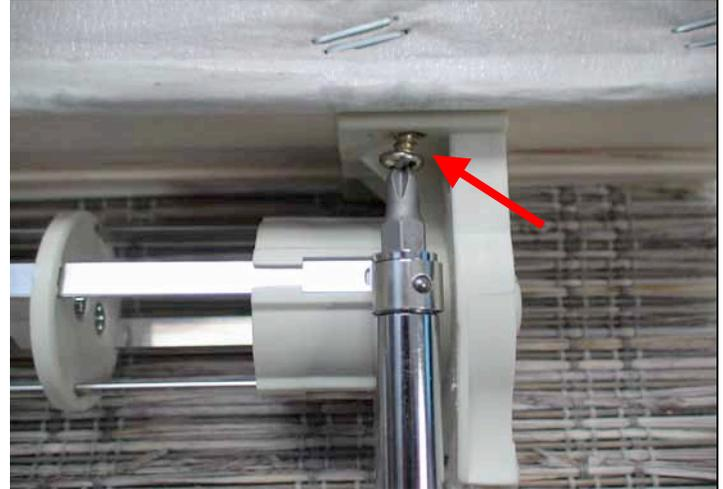
3. Remove clutch and retainer by pulling each piece in the opposite direction until the spears have completely disengaged.
