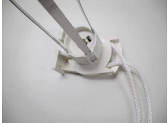
7. Slide NEW retainer into shaft.
