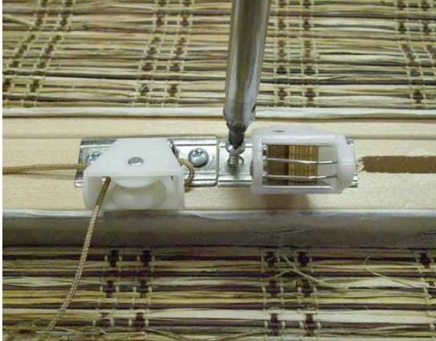
10. Thread the cords between the rollers inside the cordlock and on either side of metal cord separator.
