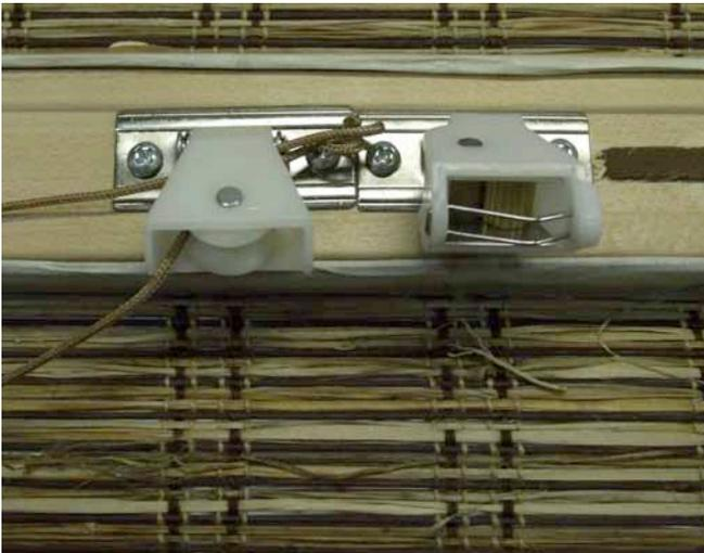
4. Remove the cordlock from the headrail by loosening the screws on each side of the cordlock.
