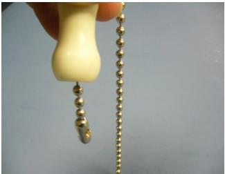
5. With louvers in the open position, and holding both pieces of chain, cut the chain between the beads at the top of the tape mark. Do not pull on the end of the chain because it can pull out of the control mechanism.
