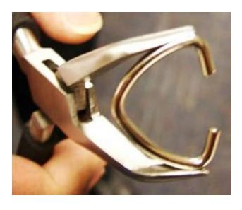
**6.** Place the open end of the "D" ring in the holes of the wand tip and squeeze the "D" ring closed.
