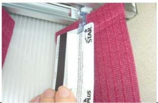
**3.** Rotate louvers stems by pulling rotation chain. If stems are rotating, turn them to the open positon. Proceed to step 7. If stems are not rotating, go to step 4.
