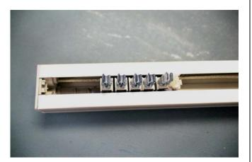
6. If you have a split stack, locate the knot holder attached to the lead carrier in the center of the blind. If you have a one-way stack, go to step 7.
