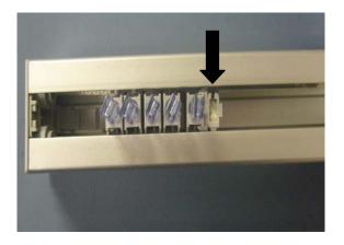
**8.** Use needle nose pliers or tweezers to grip the first knot in the knot holder and pull lightly. As the cord is pulled out through the knot holder the traverse cord will shorten.
