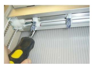
SPRINGS WINDOW FASHIONS Customer Service TASK: Only One Side of Split Stack Traverses, Gap in Center of Split Stack, Fixing Lead Carriage Connector for G85 Duralite/Duravue and G71 Supervue/Everglide Vertical Headrail Use If/When: G85 & G71 Vertical headrails - Only one side of split stack traverses, gap in center of split stack, or fixing lead carriage connector (G98 Magnum/UltraVue set screw cannot be replaced)
