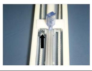
7. If the original Allen screw is still in place, manually pull the lead carriages together until they meet the spacer and tighten the Allen screw using a 1/16" Allen wrench. Pull the traverse cord to test. Both sides should now traverse
