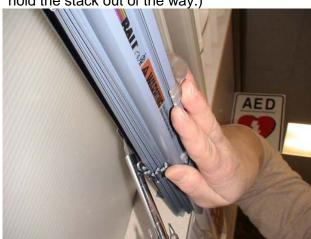
**3.** Remove dust cover, starting with top corner. Run your finger across the top. Put pressure on the back to remove.
